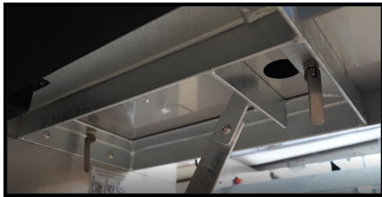
Figure 59. Unlocked conveyor cover clamping levers
