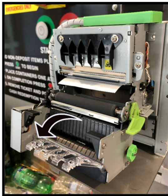
Figure 70. Printer presenter sensor cleaning
