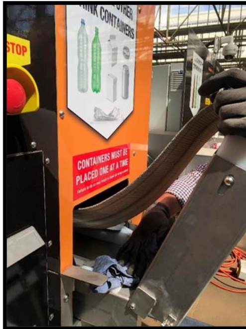
Figure 66. Conveyor Bed Cleaning
