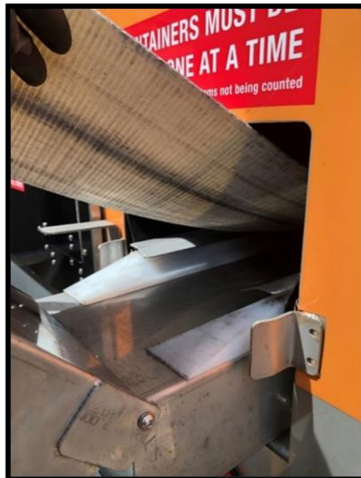
Figure 65. Belt lifted from under protection strips
