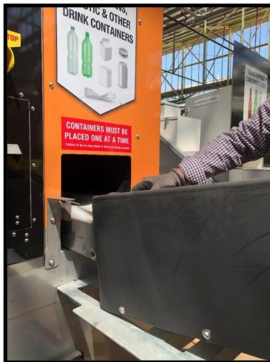
Figure 63. Lifting conveyor cover
