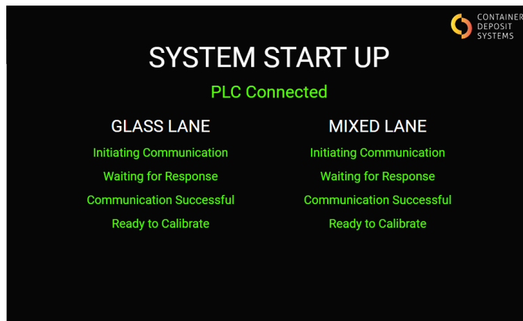
Figure 10. System Start up
