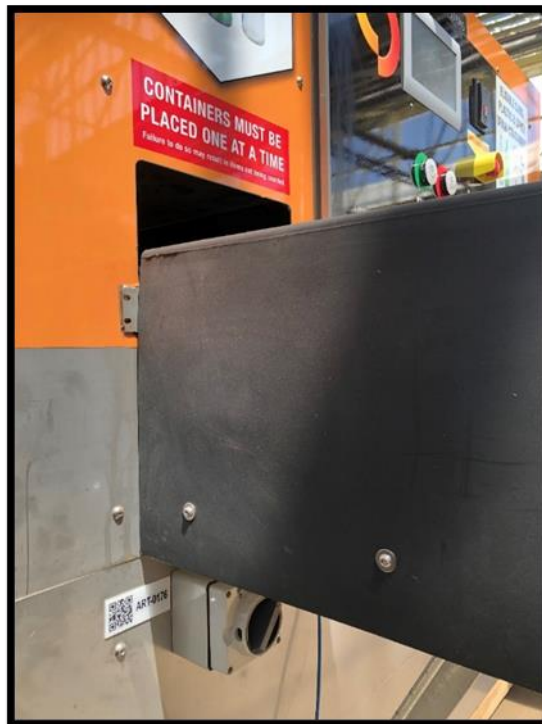
Figure 9. Power Isolator Location
