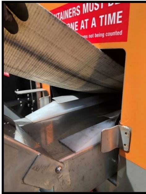
Figure 69. Belt lifted from under protection strips
