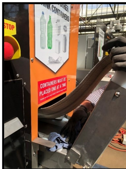
Figure 70. Conveyor Bed Cleaning
