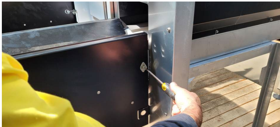
Figure 65. Locked conveyor cover
