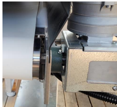
Figure 73. Greasing the Drive End Bearings
