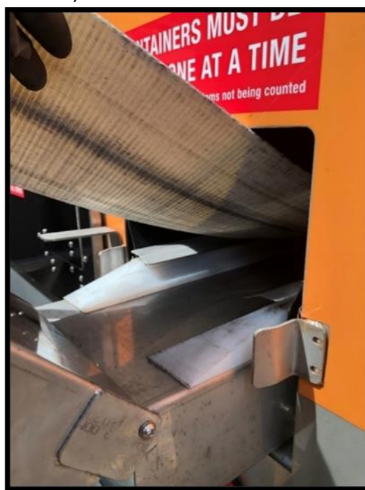
Figure 64. Belt lifted from under protection strips
