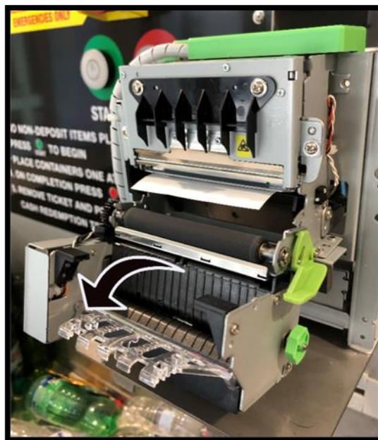
Figure 77. Printer presenter sensor cleaning
