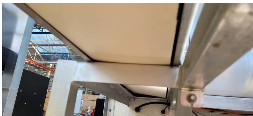
Figure 69. Incorrect belt tension
